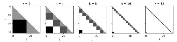
Figure 1: Comparison matrices for n=32 and different values of k. Variables i and j denote the matrix indices as used in the constraints.
