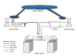
In data centers, water is consumed through **evaporation** and **blow down evaporation**  $\rightarrow$  inefficiency in chiller, **blow down**  $\rightarrow$  flush water in system Water consumption of  $\mathcal{M}$   $\rightarrow$  on-site cooling ( $W_{on}$ ) and power plant ( $W_{off}$ )
