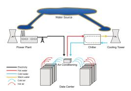
In data centers, water is consumed through **evaporation** and **blow down evaporation** → inefficiency in chiller, **blow down** → flush water in system
